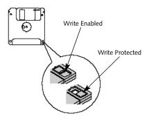
Figure 2-11 Floppy Disk Write Protect
